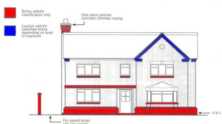
Note: Bricks with any of these ratings do not look different so ask your supplier for the rating. If bricks are not rated they should be assumed to be '0' not frost resistant. F2 products may be covered by a durability warranty however this will be invalidated if the correct design details are not applied.
